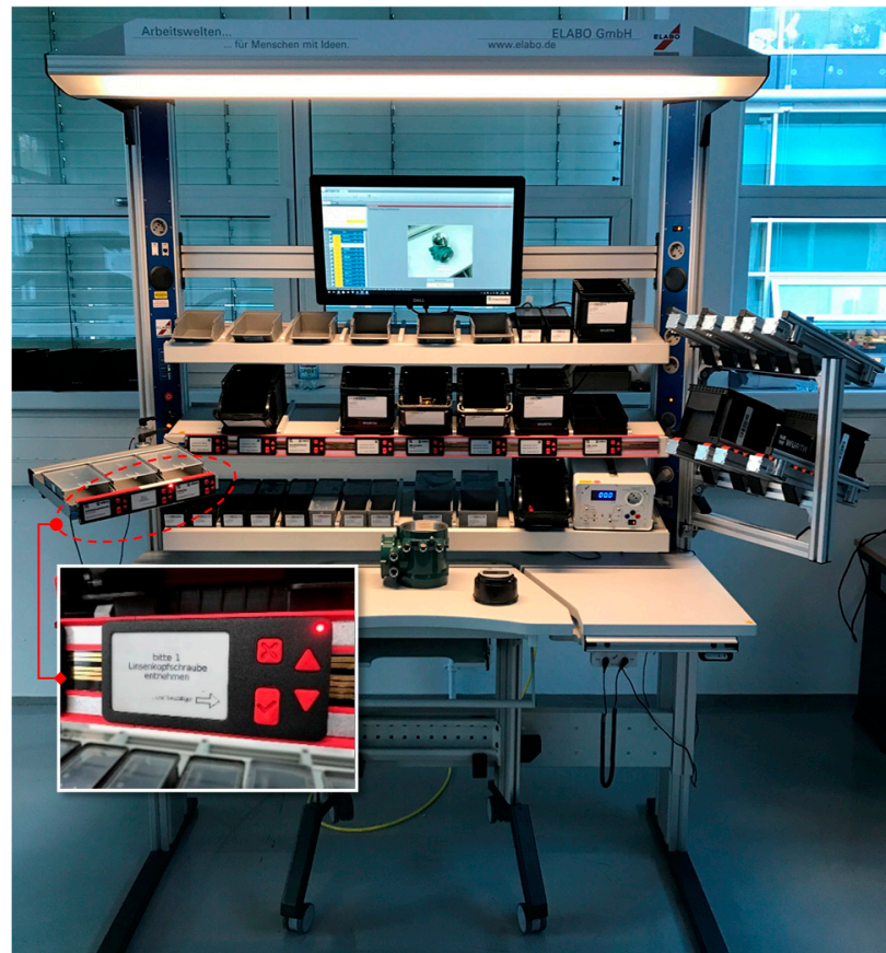
Figure 17. Prototype of the manual assembly workstation with cognitive assistance system and pick-by-display system.
