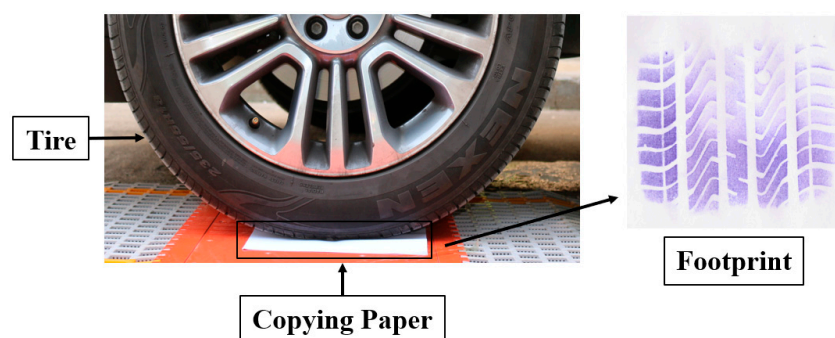
Figure 8. Test for obtaining the tire footprint.
