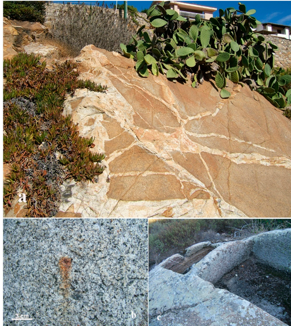
Figure 4. Chromatic alteration of the original grey colour due to oxidation phenomena in a granite outcrop at the base of Giglio Castello city walls. The white veins are the filling by quartz (a); oxidation of a pyrite crystal (b); bio-colonisation in tanks of a palmento , a traditional construction for the processing of grape must (c).
