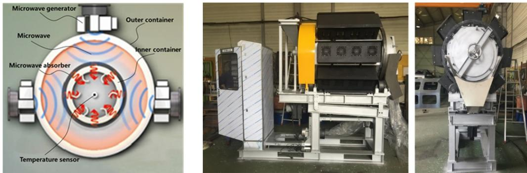
Figure 3. Indirect-heated microwave thermal desorption equipment.
