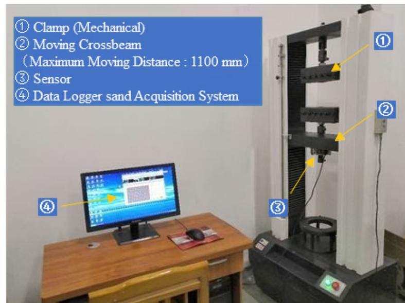
**Figure 1.** The geosynthetics electronic strength tester.
