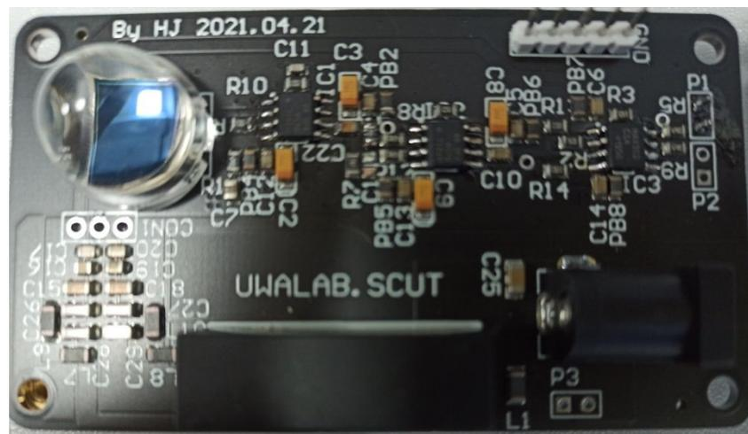
Figure 5. Visible light receiving circuit physical model.
