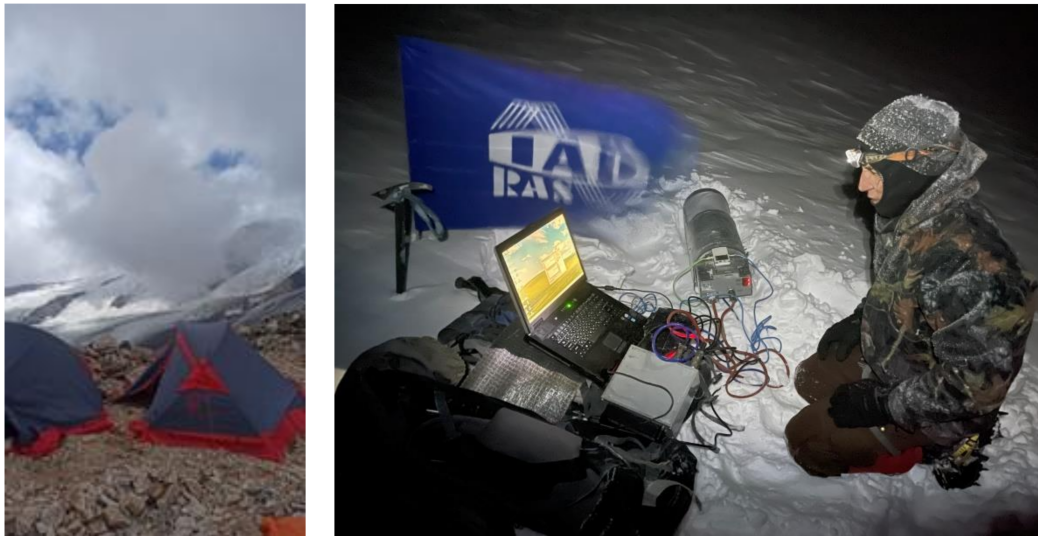
Figure 5. Elbrus IAP RAS expedition August 2021: night measurements at 5630 m made by MIAP-2. There is \sim 0.25 \pm 0.25 Np of absorption of 3 mm waves.
