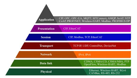
Figure 2. Communication layers and protocols.
