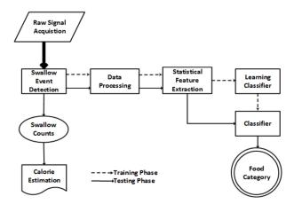
Figure 1. An overview of food intake monitoring system.
