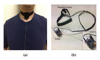
**Figure 3.** Necklace-type wearable system: (**a**) Subject wearing a necklace; (**b**) Necklace connected to Simblee.
