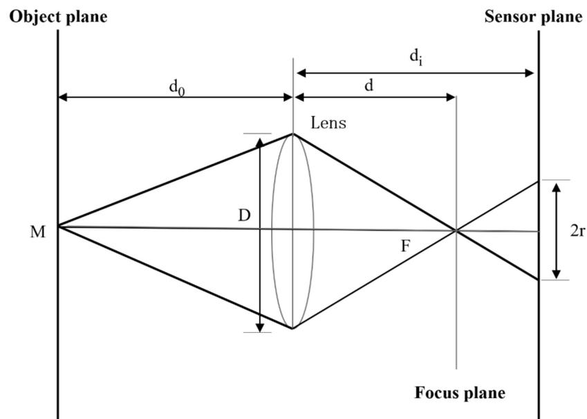
Figure 1. The basic principle of optical imaging characteristics.
