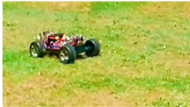
Figure A2. The straight road test on a slippery wet grass surface (captured when the speed of the rover was around 42.8 km/h.).
