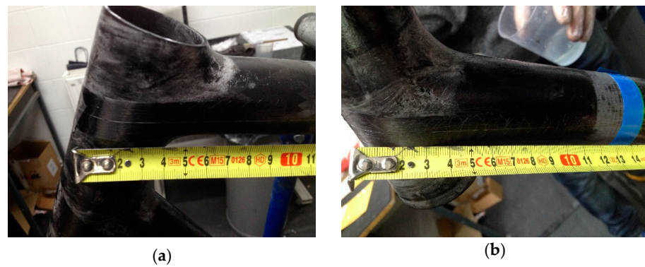
Figure 3. (a) Detail of FBG TT sensor placement during the hand lamination process; (b) Detail of FBG DT sensor placement during the hand lamination process.
