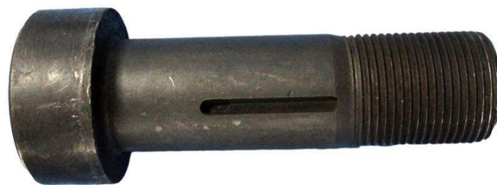
Figure 4. The M60 high-strength bolt used in this work.
