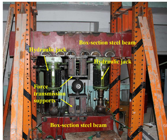
Figure 6. The fatigue testing machine and the loading device.
