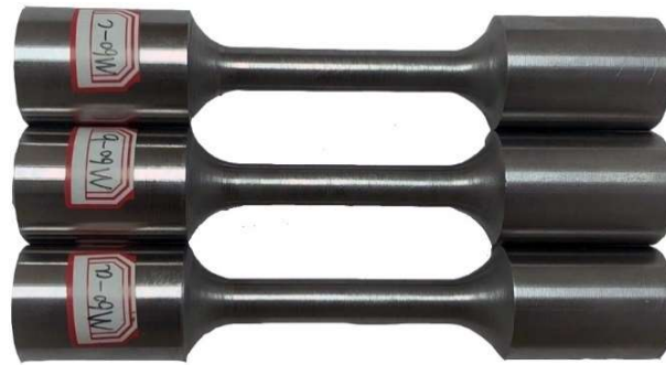
Figure 5. The standard specimens of the M60 high-strength bolt for tensile tests.
