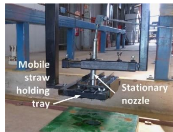
Figure 6. Bench tests of cutting wheat straw internode stem by water jet ([73], reproduced from “A laboratory evaluation of waterjet cutting of crop residue using the Aqua-Till® liquid coultter” with permission from Elsevier, 2022).
