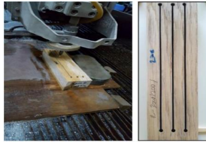
Figure 5. Cutting wood in an abrasive water jet (AWJ) system ([71], reproduced from “Influence of processing parameters on the surface roughness of solid wood cut by abrasive water jet” with permission from NC State University, 2022).
