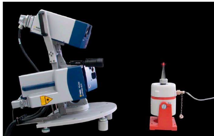
Figure 9. 3-D scanning vibrometer testing a turbine blade [121].
