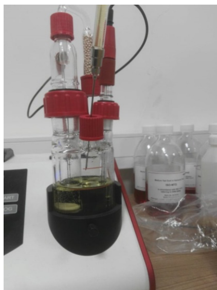
Figure 3. Tested oil with solvent and iodine on Automatic Cou-Lo AquaMax KF titrator.
