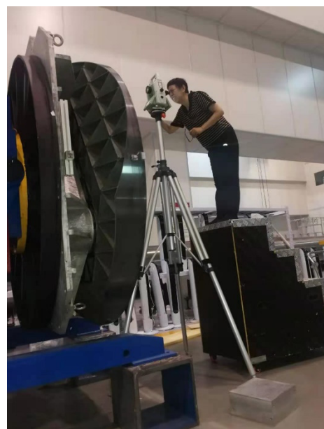
Figure 17. Detected rigid displacement and tilt angle of the mirror body using a theodolite.
