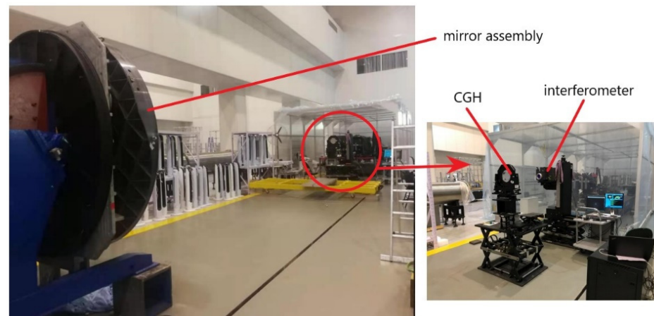
Figure 16. Detected mirror surface error using an interferometer.
