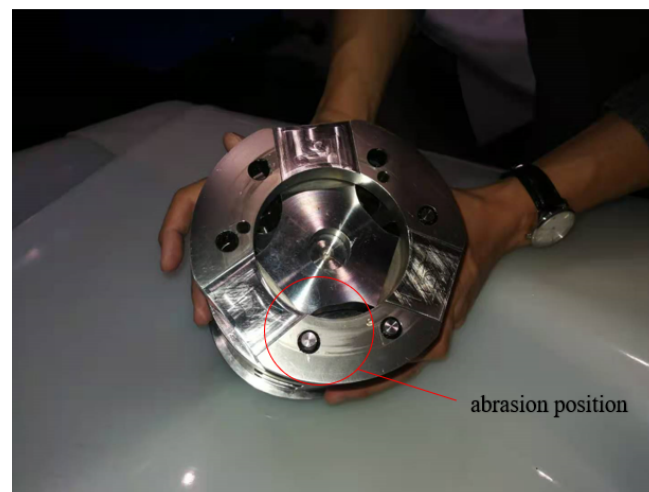
Figure 15. Abrasion of the flexible structure.
