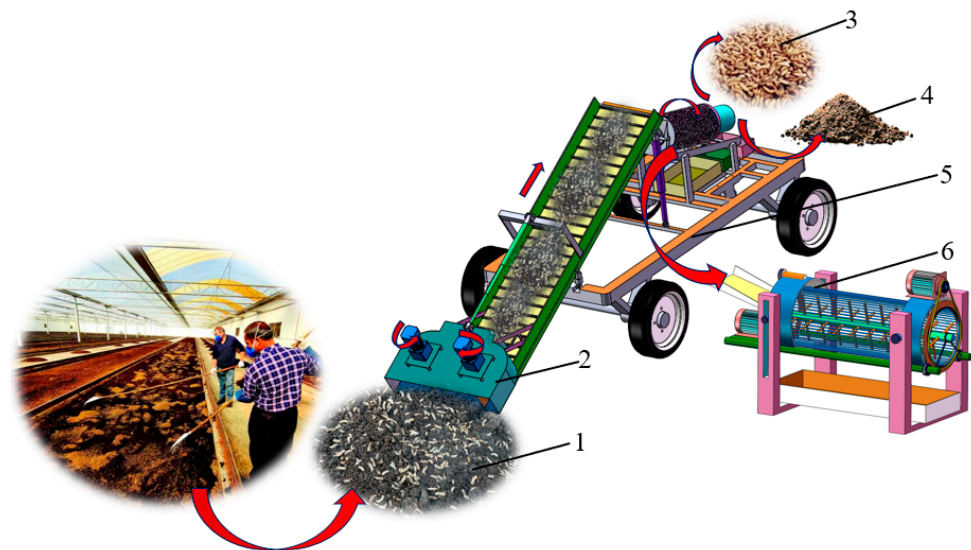
Figure 4. Structure and working principle of the ground trough BSF sand conveying and sorting machine. 1—BSF mixture; 2—parallel double-impeller collecting device; 3—BSF larvae; 4—BSF frass; 5—chassis; 6—sieve device with different rotational speeds.
