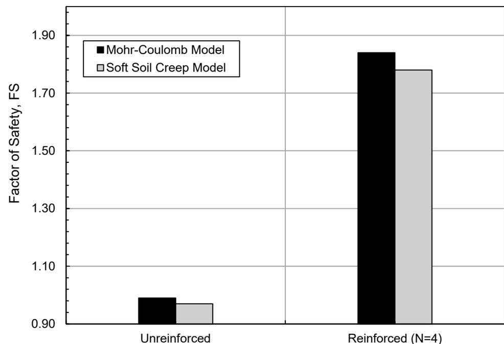
Figure 19. FS values obtained from different material models.
