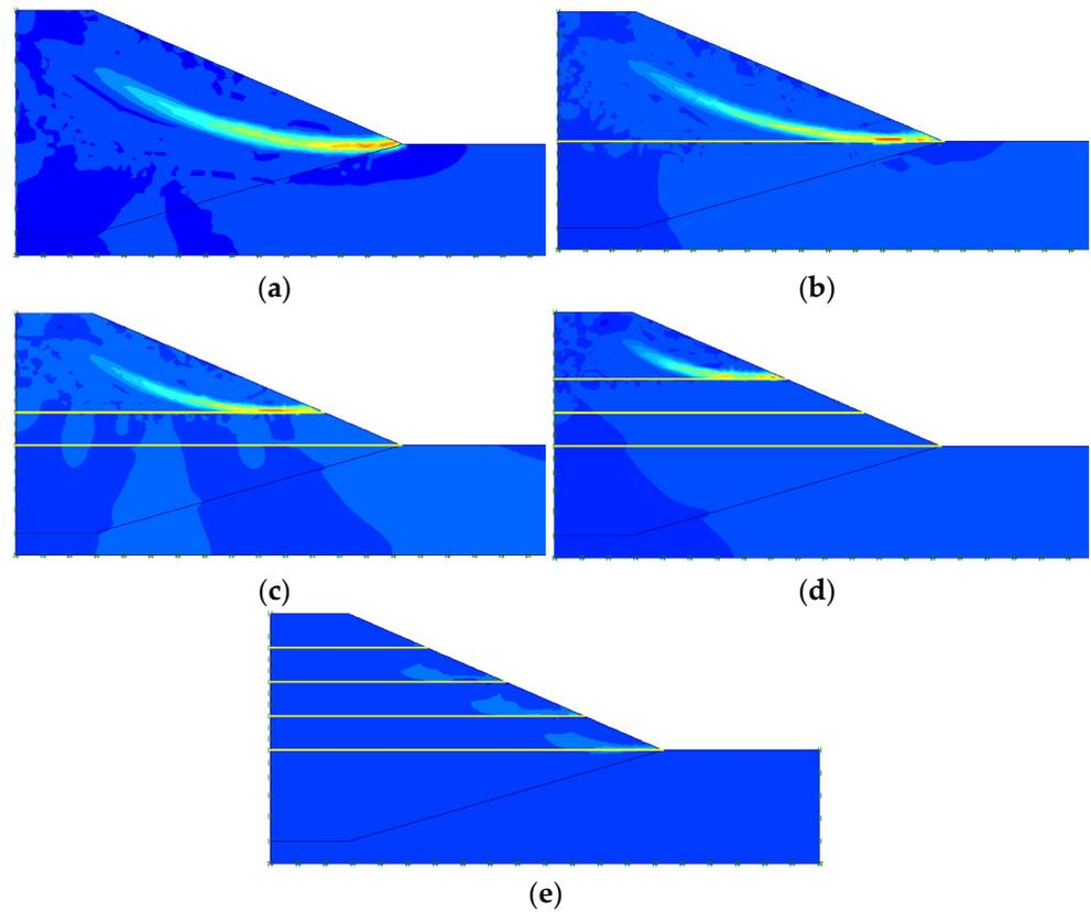
**Figure 11.** (a) Shear strain increment (without geogrids); (b) shear strain increment with one geogrid; (c) shear strain increment with two geogrids; (d) shear strain increment with three geogrids; (e) shear strain increment with four geogrids. Shear strain increment in FEM analysis.
