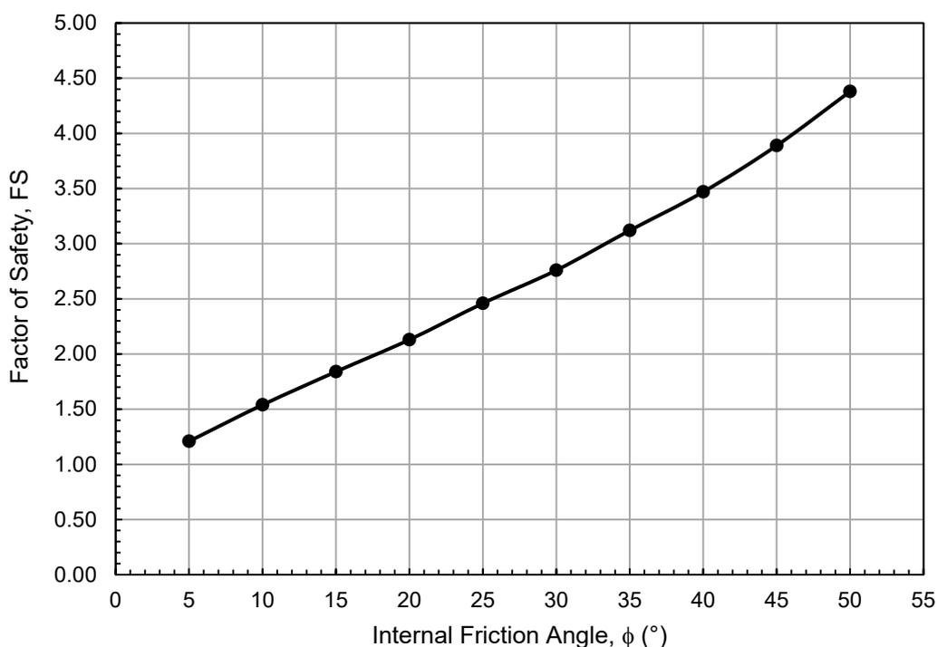
**Figure 17.** Variation in FS with  $\phi$  for the reinforced slope.
