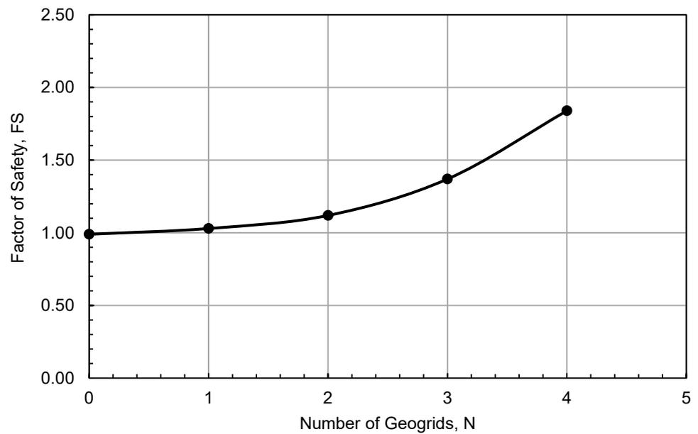
**Figure 12.** Variation in FS with N (1V/2H slope) (FEM).
