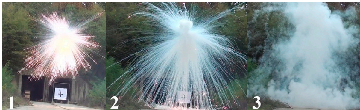
Figure 2. Three-step smoke screen formation: 1—PC1 combustion, instant smoke screen; 2—PC2 and PC3 combustion, smoke screen formation; 3—PC3 continue to supply the smoke screen.
