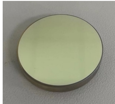
Figure 3. The superpolished sample with reflective silver-enhanced coating.
