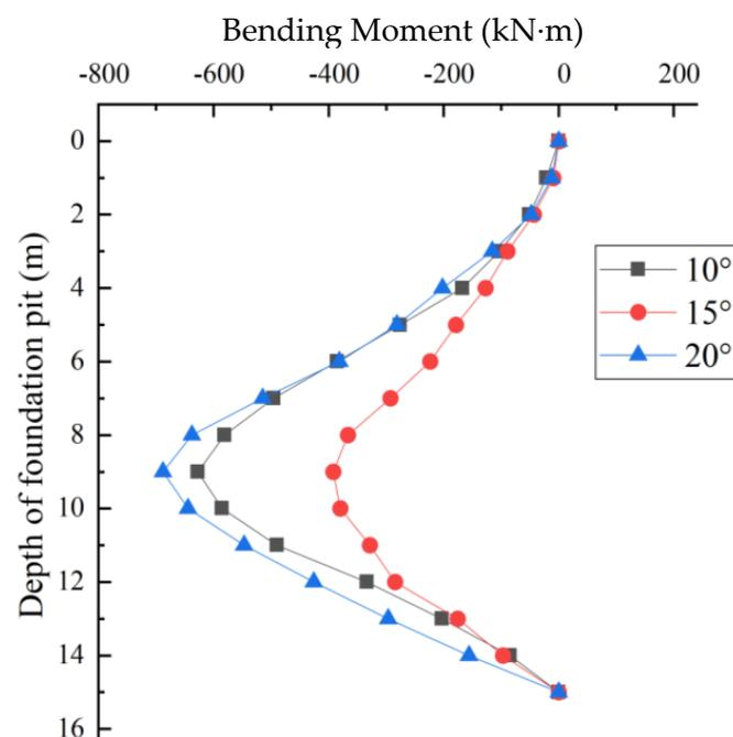
Figure 16. Pile bending moments.
