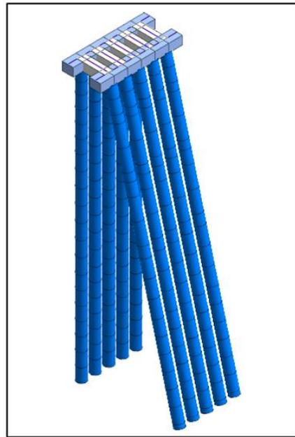
Figure 2. Sketch of the double-row pile.
