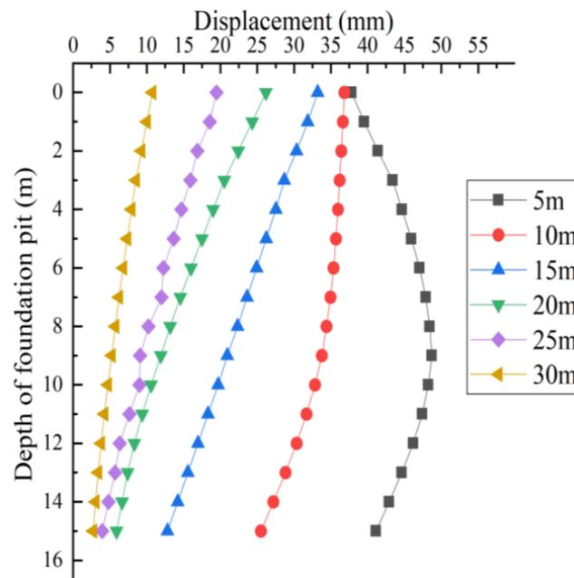
**Figure 13.** Pile displacement behavior.
