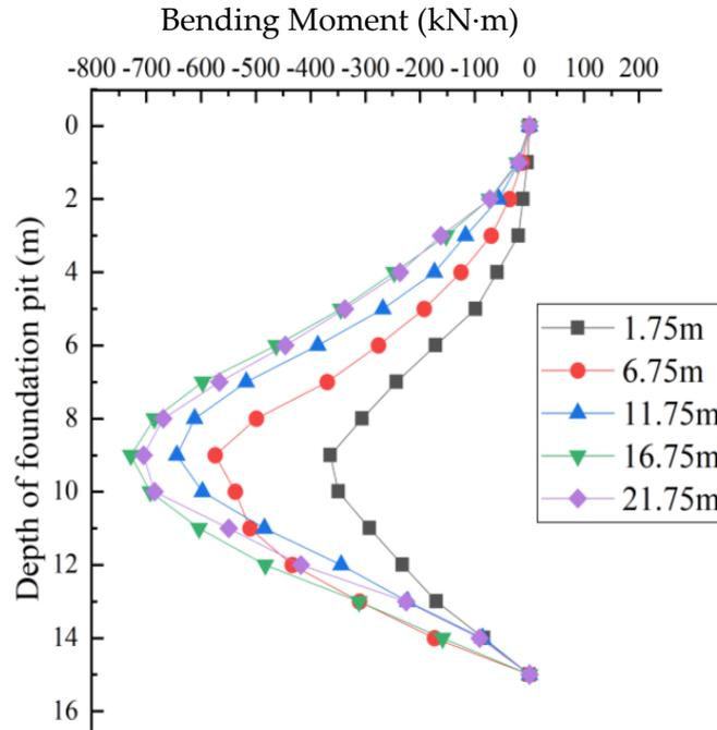
Figure 14. Pile bending moments.
