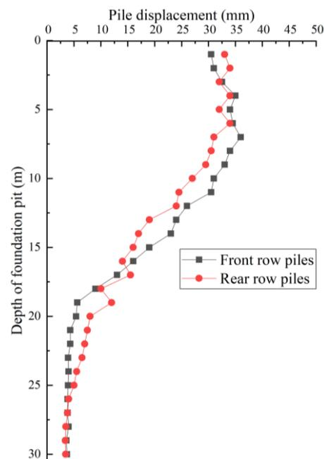
Figure 10. Horizontal displacement of front and rear rows of piles.
