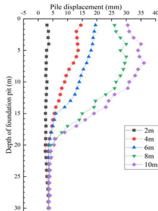
Figure 9. Horizontal displacement of front row inclined pile.
