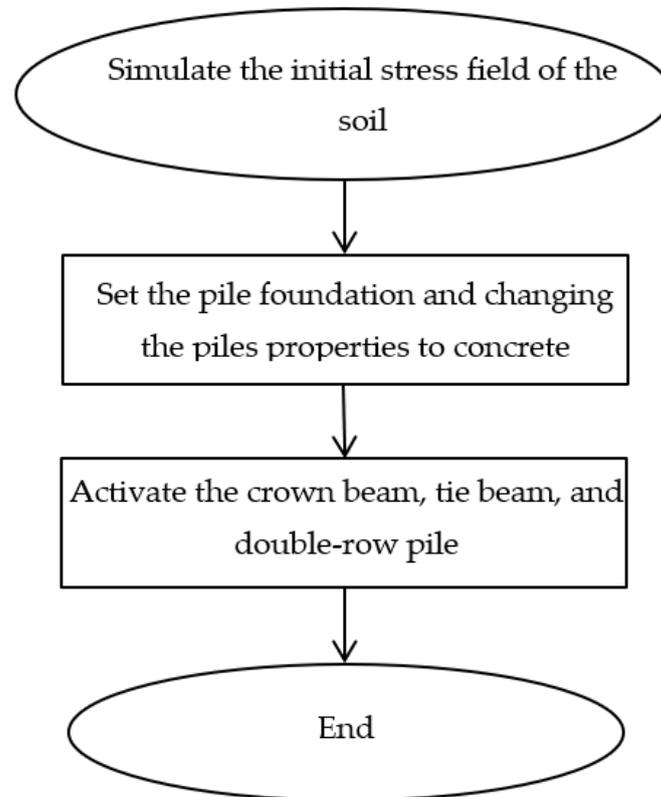
Figure 5. Construction stages flowchart.
