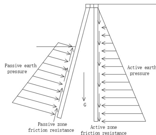
Figure 11. The behavior of force analysis of inclined-straight pile. Where, (G is the gravity of soil between combined piles).
