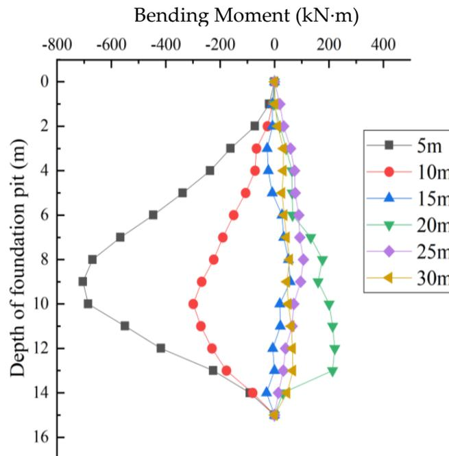
**Figure 12.** Pile bending moments.
