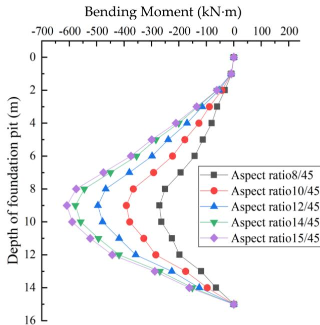
Figure 18. Pile bending moments.
