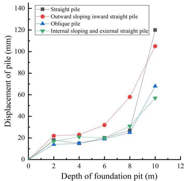
**Figure 1.** Variation of displacement of row pile under different working conditions.
