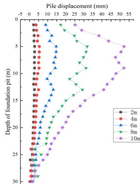
Figure 7. Horizontal displacement of rear straight pile.
