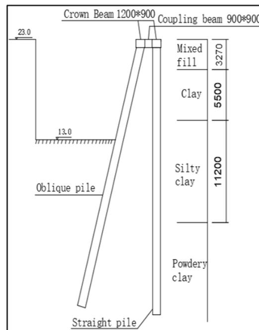
Figure 3. Layout of Foundation pit section. (unit: mm).
