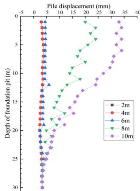
Figure 8. Horizontal displacement of rear straight pile.
