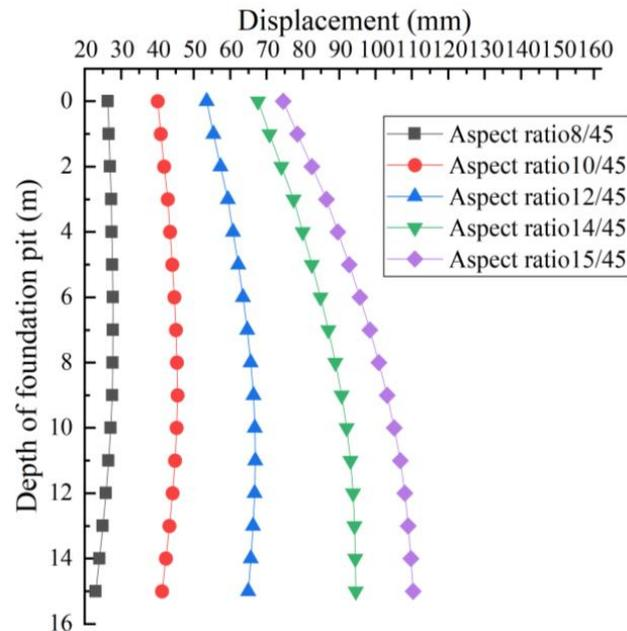
Figure 19. Pile displacement behavior.
