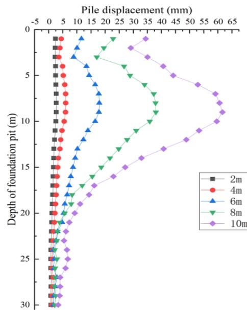
Figure 6. Horizontal displacement of front row inclined pile.
