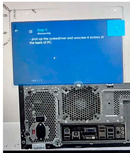
Figure 7. Virtual image in the HoloLens 2 showing both the text explanation to unscrew the power supply unit and the highlighted (dotted circles) screws to be unscrewed and removed (step 5 of disassembly task).
