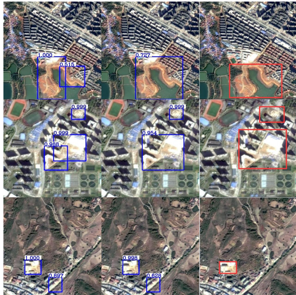
Figure 7. Detection results of the Faster RCNN method and this method. Each row in the figure is from the same image as a group for detection. From left to right, the purple candidate boxes in the first and second columns are detection results of Faster RCNN and this method respectively, and the red boxes in the third column are ground truth.
