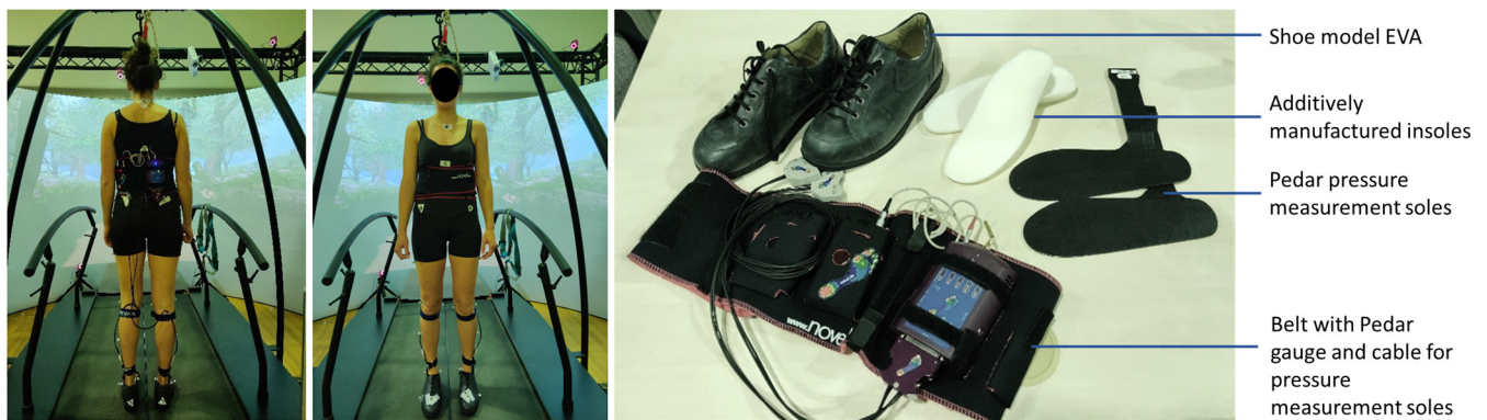
Figure 1. Experimental setup of the 3D gait analysis using Gait Realtime Analysis Interactive Lab and the attached reflective markers and Pedar pressure measurement insole system.
