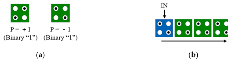
Figure 1. Two polarization states of the QCA basic cell: (a) P = +1 (binary 1), P = -1 (binary 0); (b) QCA cell-based wiring.
