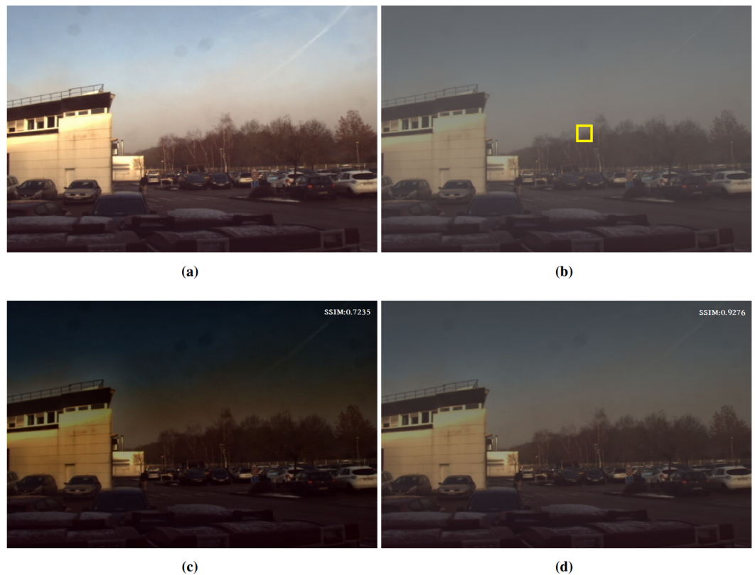
Figure 14. Dehazing result using PolarLITIS dataset image. (a) Real image. (b) Foggy image. (c) Result using original DCP. (d) Result using the proposed approach.
