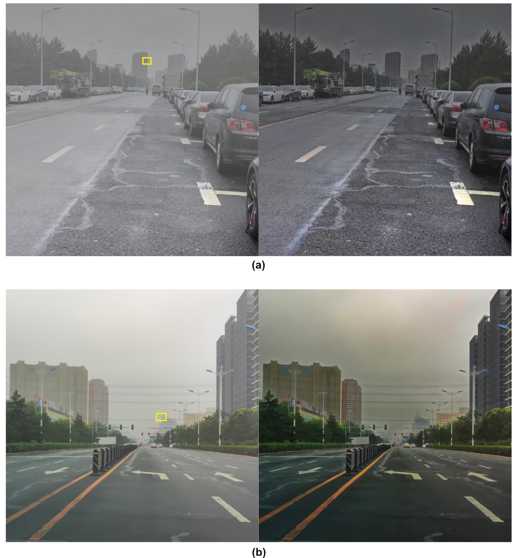
Figure 13. Dehazing effect on rainy weather and smoggy weather image. (a) The dehazing effect on images captured during rainy weather. (b) The dehazing effect on images captured during smoggy weather.
