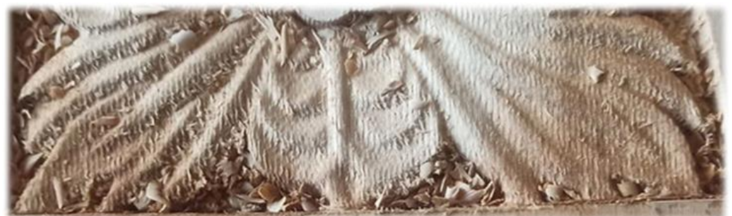
Figure 4. Detailed view of the CNC machining process of the lime wood.
