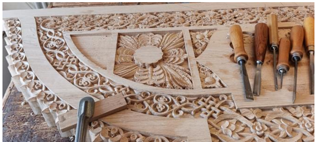
Figure 6. Refinement of the wood-carving in the lime wood after applying handiwork by wood-carvers.
