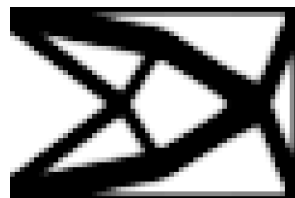
Figure 15. Structure obtained using the traditional equally weighted sum (TEWS) method (Stage 1) and the bisection constraint method (BCM) for Problem 1 with F_1 = 1.0 and F_2 = 1.0 (same result).
