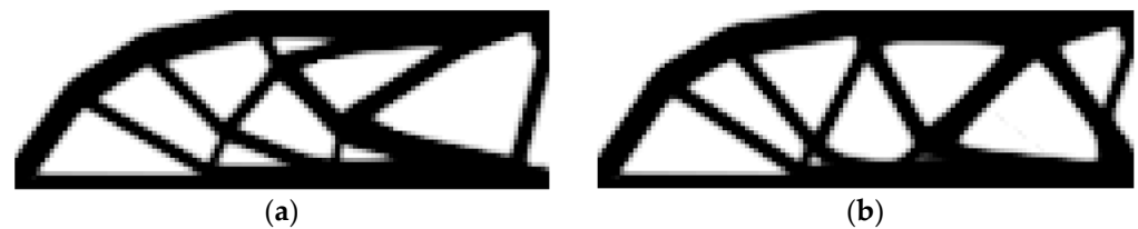
Figure 7. Topologies in Case Study 2: (a) after Stage 1 (traditional equally weighted Sum method); (b) after Stage 2.
