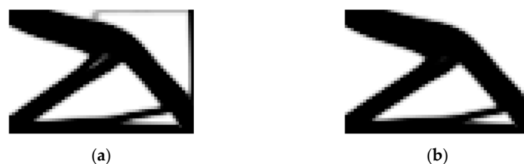
Figure 10. Structures obtained in Problem 1 with F_1 = 0.2 and F_2 = 1.0 : (a) after Stage 1 (traditional equally weighted sum method); (b) after Stage 2.
