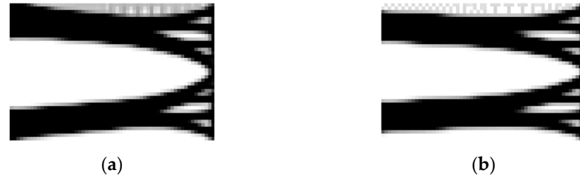
Figure 18. Obtained structures for Problem 2 when P_1 = 0.5 and P_2 = 9.5 : (a) using the traditional equally weighted sum method; (b) using the bisection constraint method.
