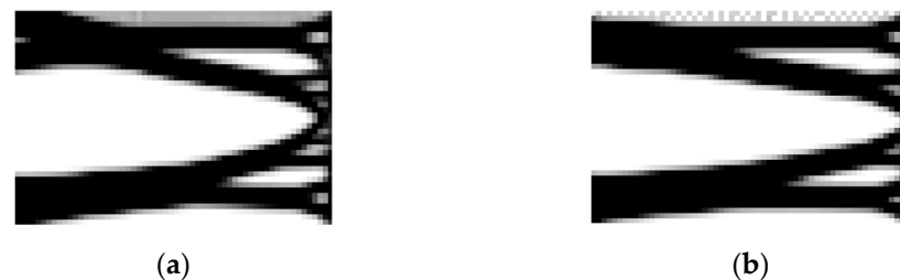
Figure 20. Structures obtained in Problem 2 when P_1 = 1.0 and P_2 = 9.0 : (a) using the traditional equally weighted sum method; (b) using the bisection constraint method.
