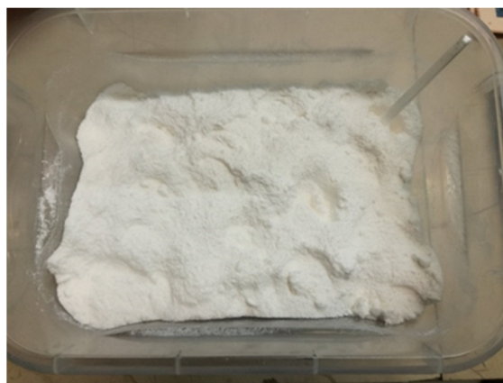
Figure 1. Appearance of ground ammonium nitrate.
