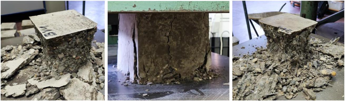
**Figure 5.** Concrete cubes after the compression test: unreinforced cube BV1 (left); fiber-reinforced cube ZV1 after the compression test (center); and fiber-reinforced cube ZV1 after the compression test and removal of the cracked parts by hand (right).
