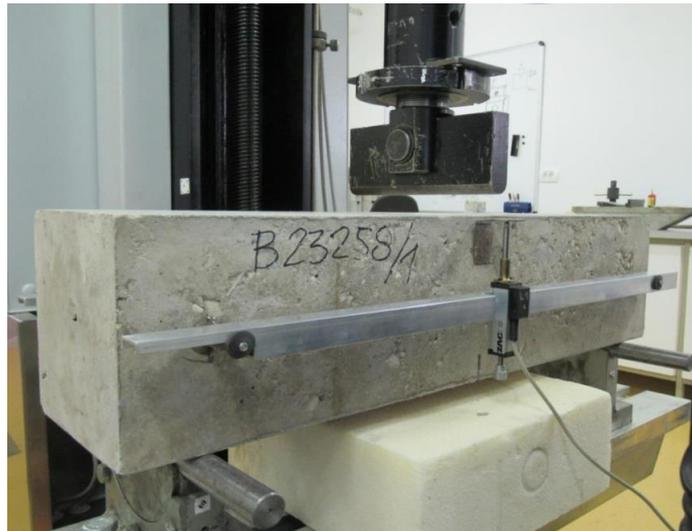
**Figure 1.** Three-point bending test configuration (the specimen B23258/1 is shown).
