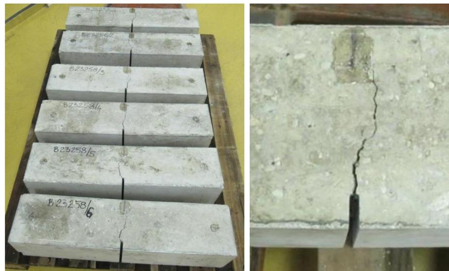
**Figure 4.** Fiber-reinforced prisms after bending tests (left) and the notched region (right) with the crack after the bending test (prism B23258/1).
