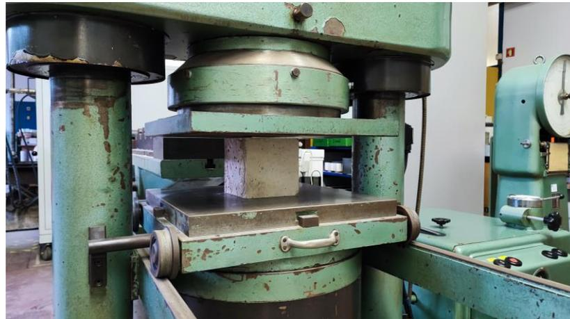
**Figure 2.** Compression test.
