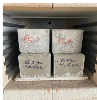
Figure 21. View of the PCC and 5% fiber sample before testing at 600 °C.
