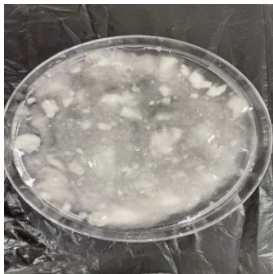
Figure 4. The ceramic fiber soluble in Na 2 SiO 3 .
