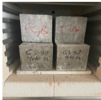
Figure 23. View of the PCC and 10% fiber sample before testing at 900 °C.
