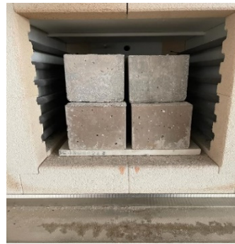
Figure 22. View of the PCC and 5% fiber sample after testing at 600 °C.
