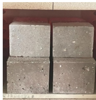
Figure 24. View of the PCC and 10% fiber sample after testing at 900 °C.
