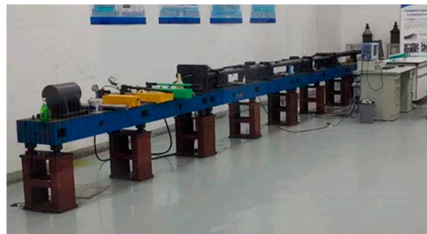
Figure 2. Dynamic and static combination SHPB test device.
