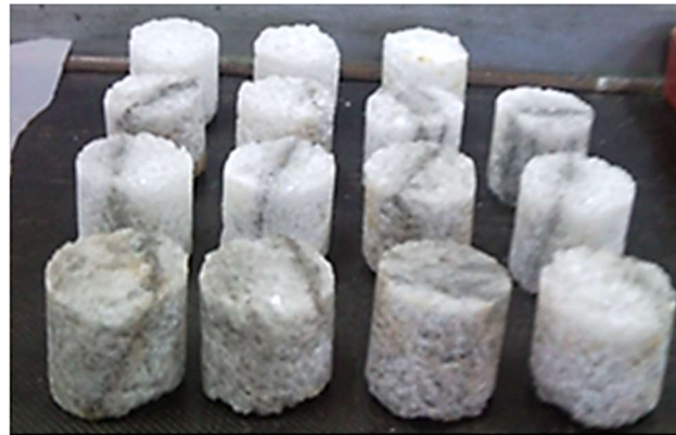
Figure 1. Salt samples were used to determine the geomechanical characteristics through laboratory tests [11].
