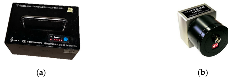
Figure 2. Instruments of measurement. (a) JM3873 system; (b) 941B accelerometer.
