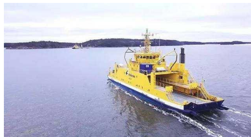
Figure 1. The autonomous ferry “Falco”.
