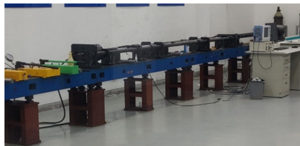
(a). Combination of dynamic and static SHPB test set: physical drawing.
