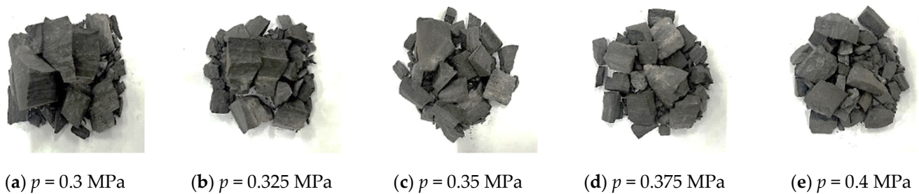
Figure 12. Impact fracture morphology of prefabricated fractured sandstone samples.
