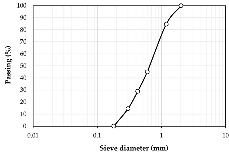
Figure 3. Grain size distribution curve of the sand sample.
