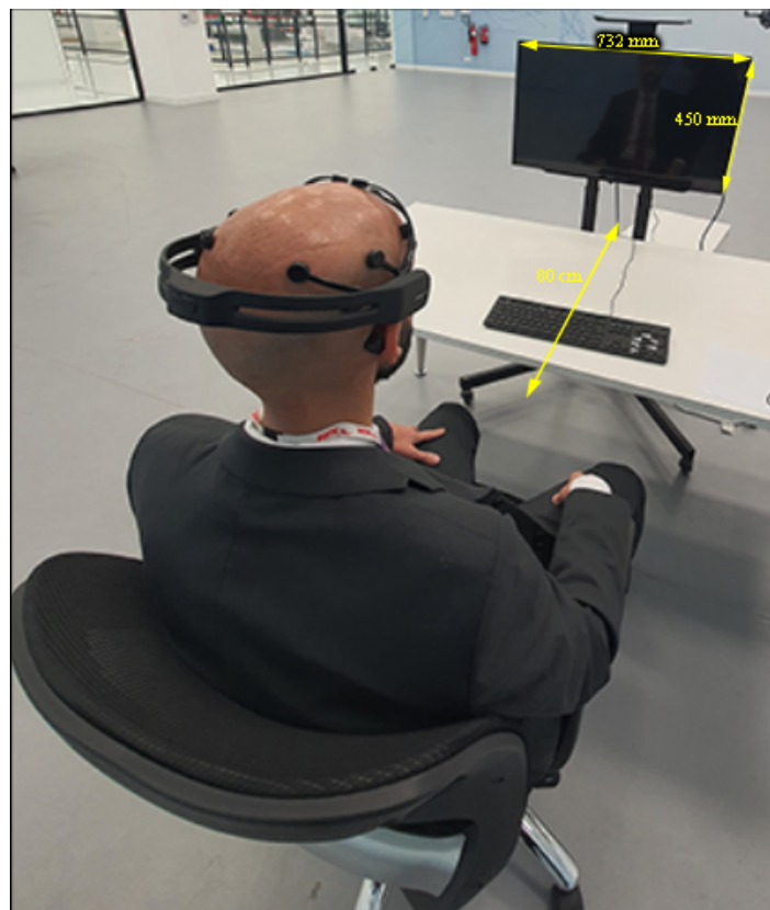
Figure 5. Full experimental setup example showing the screen dimensions and the distance between the participant and the screen.
