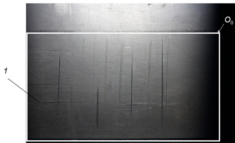
Figure 3. Specimen image obtained with the Canon EOS 1300D camera: 1—the image area for which the illumination was calculated; O_0 —the starting point of reference of conventional coordinates.
