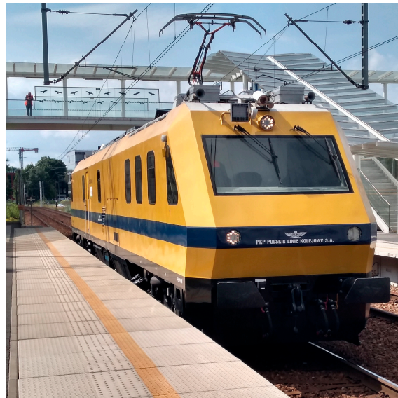
Figure 2. Track inspection vehicle managed by Polish railway lines.
