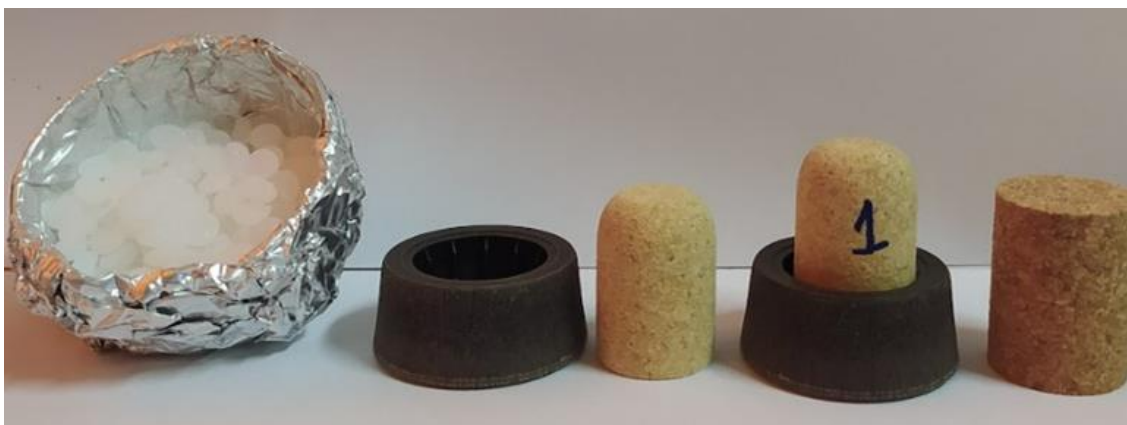
Figure 4. Elements used to perform the adhesion test. The cork samples named as 1 are bevelled and the others cylindrical.
