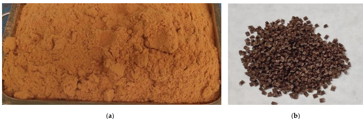
Figure 2. Physical appearance of (a) dry CoP before mixing; (b) CoP30PP70 CAG formed with a 3 mm size.
