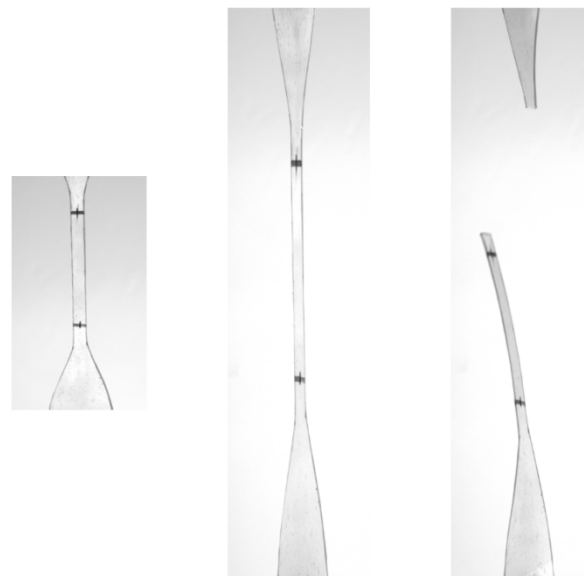
(a)Before stretching (b) 1s before fracture (c) 1s after fracture
