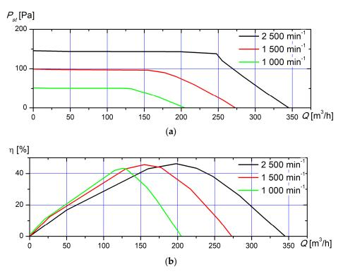
**Figure 8.** Operating parameters of optimized impeller at 2nd design point (DP): (a) performance; (b) static efficiency.
