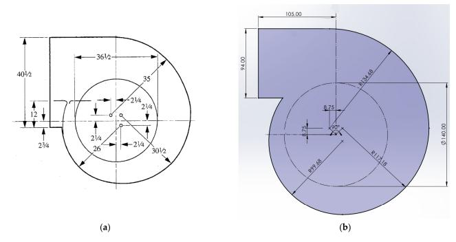
**Figure 1.** The geometry of (**a**) is a typical example, and (**b**) represents the fan used in this work. (**a**) Typical 36.5-inch impeller body (Bleier [23,24]) (measurements presented in inches); (**b**) perimeter of the case model developed for the 140 mm impeller (measurements presented in mm).
