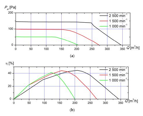
**Figure 7.** Operating parameters of optimized impeller at 1st design point (DP:) (a) performance; (b) static efficiency.
