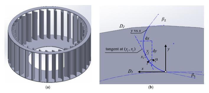
Figure 2. Fan blade geometry: (a) 3D model; (b) blade geometry design variables.
