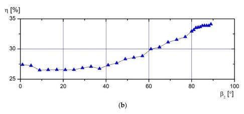
**Figure 5.** Leading- and trailing-angle influence on full efficiency at 1st design point (DP): (a) influence of angle  $\beta_1$ ; (b) influence of angle  $\beta_2$ .
