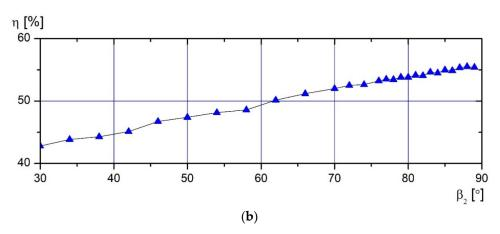
**Figure 6.** Leading- and trailing-angle influence on full efficiency at 2nd design point (DP): (**a**) influence of angle  $\beta_1$ ; (**b**) influence of angle  $\beta_2$ .
