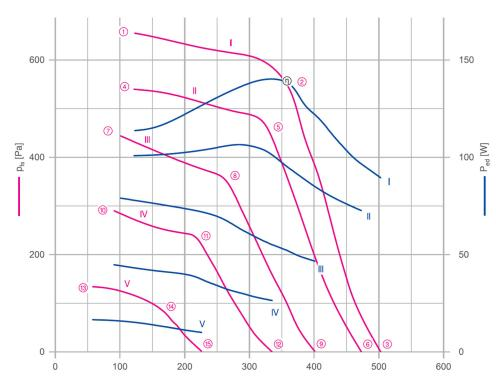
**Figure 3.** Typical performance curves given in the ANSI/AMCA 210-16 standard: I—dependence of power consumption on flow rate; II—dependence of total pressure on flow rate; III—static pressure change from discharge; IV—dependence of full efficiency on debit; V—dependence of static efficiency on debit. Here reference points are numbered from 1 to 15.
