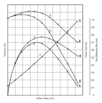
**Figure 4.** "RG14R-4IO.Z8.4R" performance curves of a centrifugal fan (Ziehl-Abegg SE [22]). Here reference curves are numbered from 1 to 5.
