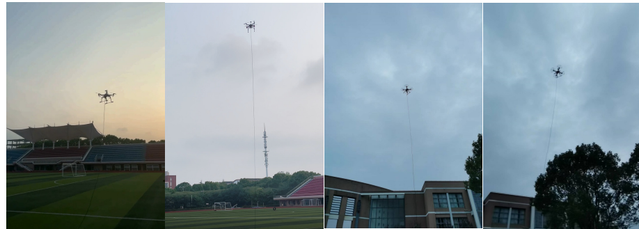
Figure 12. Real-life flight test of a tethered UAV.
