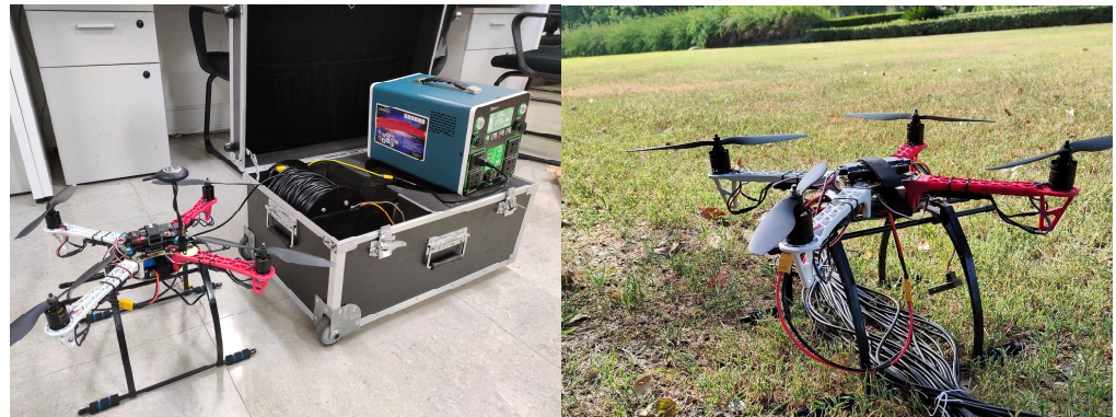
Figure 7. Physical drawing of the tethered UAV prototype.
