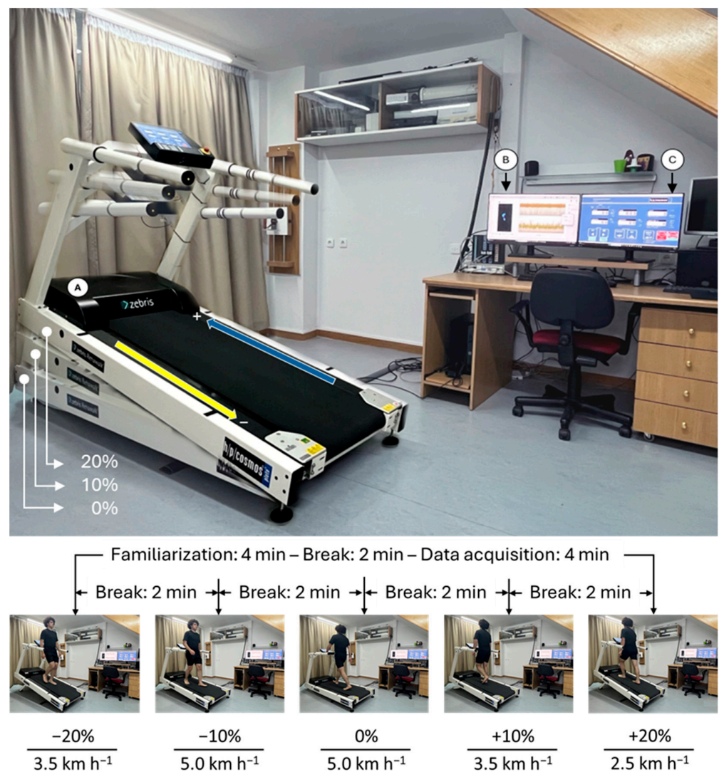
Figure 1. Experimental setup utilized in the research protocol: The treadmill's surface (A) configured for level walking (0%) with 5.0 \text{ km h}^{-1} , uphill walking on +10% and +20% slopes with 3.5 \text{ km h}^{-1} , and 2.5 \text{ km h}^{-1} , respectively, and downhill walking on −10% and −20% slopes with 5.0 \text{ km h}^{-1} and 3.5 \text{ km h}^{-1} , respectively. Display on the screen of the data transferred to the desktop (B) and the software provided by the manufacturer (C) for remote control of the treadmill.
