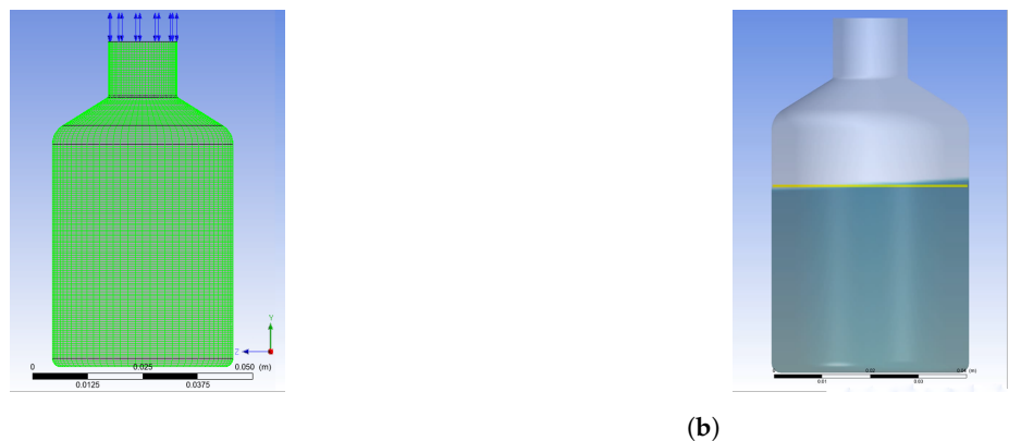
Figure 3. Glass vial mesh in Ansys Fluent (a) and water volume fraction during oscillations in a simulation (b).
