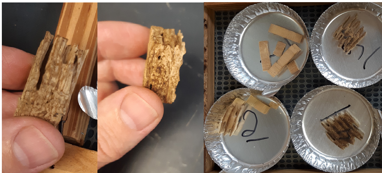
Figure 6. Photos of in-situ wood strand-based (WSB) specimen (far left) with slight to moderate damage; WSB control specimen (middle image) with slight to moderate damage; and solid southern yellow pine (SYP) wood control specimens (far right) with very severe 50–75% and up to 100% complete failure of termite attack by subterranean termites ( Reticulitermes flavipes ) during a 28-day-long American Wood Protection Association (AWPA) E1-23 termite test.
