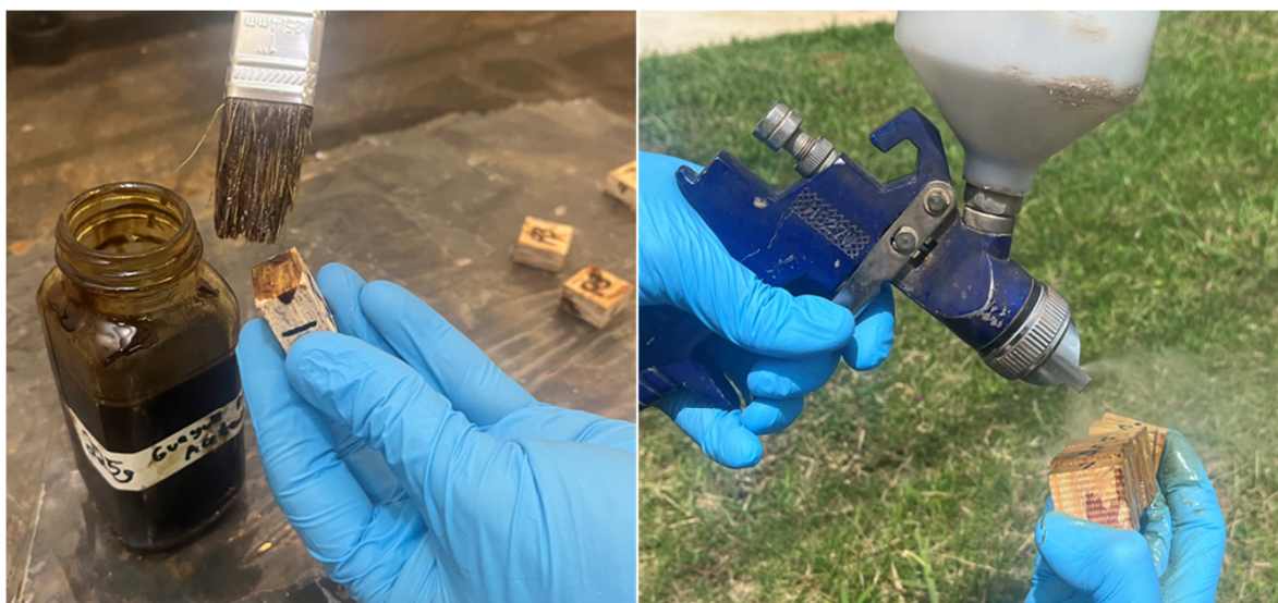
Figure 2. Brushing (left image), using a 2.54 cm wide paint brush, versus spraying (right image), using a gravity feed air spray gun, techniques with a uniform guayule–acetone solution to treat wood strand-based (WSB) panel specimens prior to testing.
