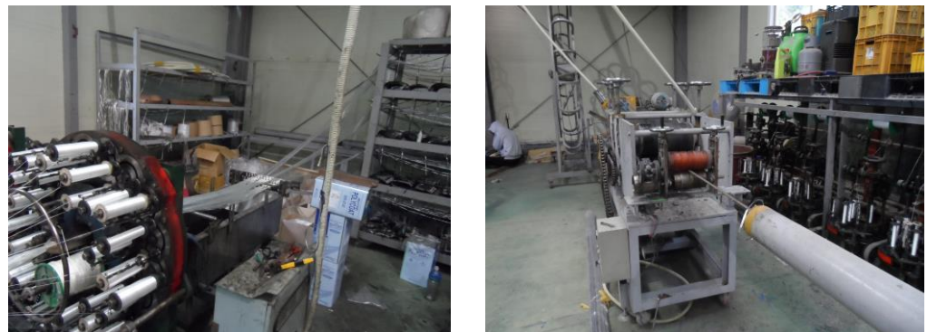
Figure 1. Fabrication of a GFRP hybrid rebar prototype using the pultrusion method.
