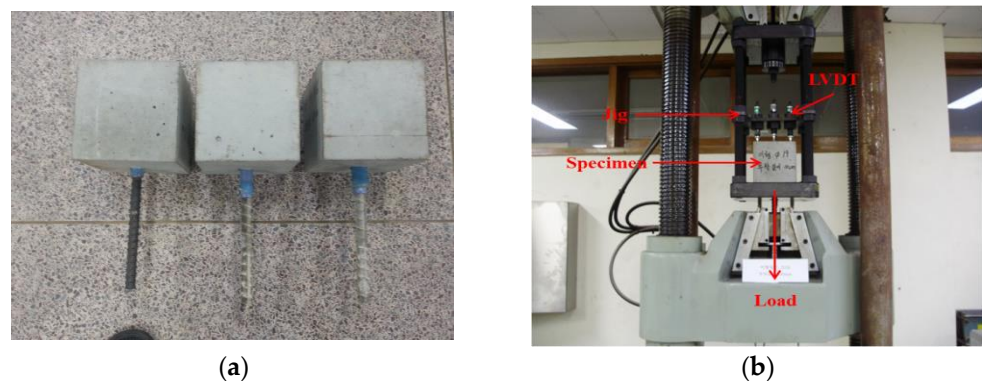
Figure 5. GFRP hybrid rebar specimens and experiment setup [2]. (a) GFRP hybrid rebar specimens; (b) Experiment setup.
