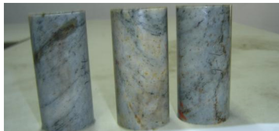
Figure 1. Photos of some rock samples before the freeze–thaw experiment.
